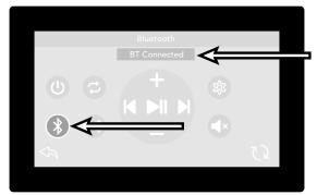
**IMPORTANT:** When your spa loses power, all paired devices are erased from the bba3 amplifier's memory. An error message may appear if your smart device still remembers the bba3 amplifier when trying to reconnect in this situation. You may need to force your smart device to "forget" the bba3 amplifier, then connect to the bba3 amplifier again to avoid the error messages.
