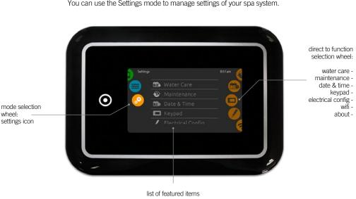
To select the settings mode, slide the left wheel up or down until the settings icon menu is highlighted in the middle.
