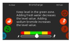
To perform a water test, slide the right wheel until the add BromiCharge^m icon is highlighted in the middle.
